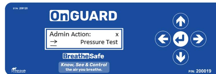
3. It is critically important that the cabin door and windows are fully **closed** during this operation. If the Minimum Pressure percentage is not reached, a Test Failure alert is raised.
