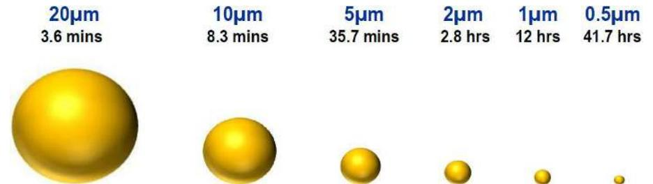
Warehouses and workshops do not have still air, so hazardous airborne particulates may remain in air for longer, increasing chance for workers to breathe in dust. Ensure PPE is worn when installing this system.
