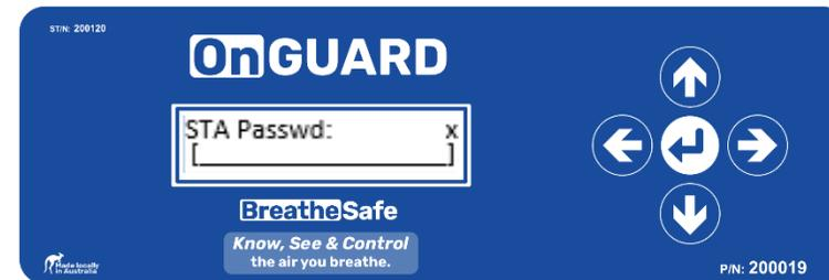
8. Select the addressing type by cycling through the options with the up (↑) and down (↓) buttons. The default option is dhcp and is standard for most networks. Consult your network admin to confirm the configuration of the network being connected to.
