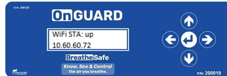
17. The IP address displayed (10.60.60.72 in the example) is the address of the OnGuard web interface on the network. Navigate to this address via a web browser on a device connected to the same network to access the OnGuard's web interface.
