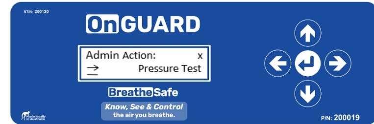
3. It is critically important that the cabin door and windows are fully **closed** during this operation. If the Minimum Pressure percentage is not reached, a Test Failure alert is raised.
