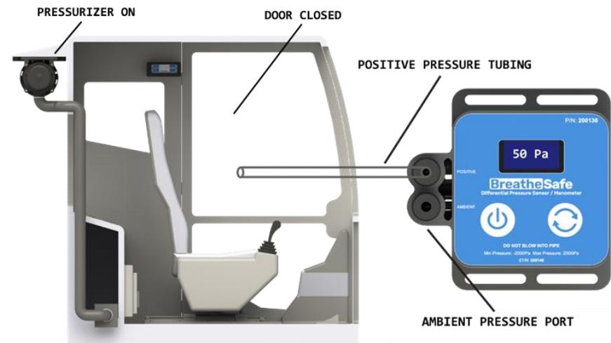
Sensor Outside the Cabin: Attach pressure tubing to the **positive** pressure port and place the other end of the pressure tube inside of the cabin.
