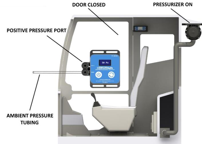
Sensor Inside the Cabin: Attach pressure tubing to the **ambient** pressure port and place the other end of the pressure tube outside of the cabin.
