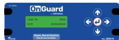
Cabin sealing needs to be checked and improved if maximum pressure is below 250 Pa with a new filter. Cancel the test by pressing the centre 'enter' button.
