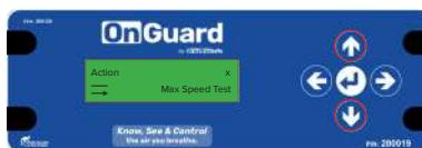
Press the 'up' or 'down' buttons to navigate to "Max Speed Test". Begin the test by pressing the 'enter' button.
