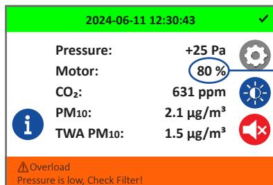
Ensure doors and windows are fully closed, allow unit to enter normal operation. Replace filter if pressure is below target (default 50 Pa) or motor speed is at or above 80%.
