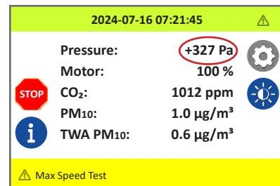
Cabin sealing needs to be checked and improved if maximum pressure is below 250 Pa with a new filter.
