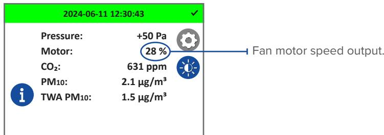
BreatheSafe recommends OEM air conditioning fan is set at mid-speed or greater to circulate air around the breathing zone and minimise CO<sub>2</sub>.
