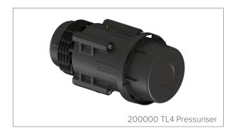
BreatheSafe's High Pressure Air Filtration Unit (HPAFU) precleans, filters and pressurises external air delivered to enclosures. Utilising a IP66 rated, variable speed, brushless, DC motor, this system is engineered for longevity under extreme conditions. The unit houses an easily serviceable HEPA H14 filter and mechanical pre-cleaner for removing large particulate from the incoming airflow to provide long service life on every filter.
