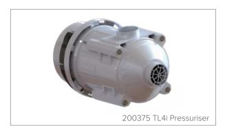
BreatheSafe's High Pressure Air Filtration Unit (HPAFU) filters and pressurises external air delivered to enclosures. Utilising a IP66 rated, variable speed, brushless, DC motor, this system is engineered for longevity under extreme conditions. The unit houses an easily serviceable HEPA H14 filter.
