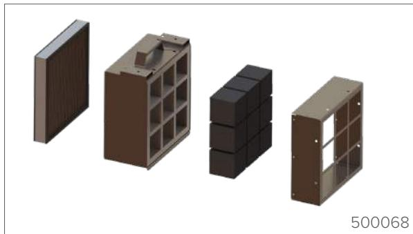
Two-stage Activated Carbon + HEPA filter assembly. Specially designed to minimise air velocity and maximise contact surface area of the reactive carbon, promoting gas filtration effectiveness. Provided with custom designed assemblies to integrate gas filtration with BreatheSafe pressurisation systems. Cartridge is self-contained and easily swapped during scheduled machine maintenance.
