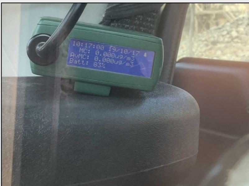
The test result must be zero mass concentration (MC)
