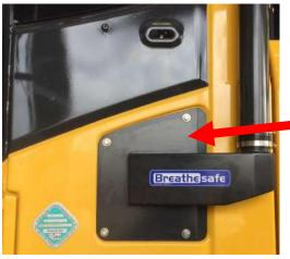
Fit an inlet spigot or custom duct to introduce the hepa filtered air into the HVAC.
