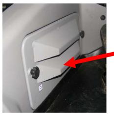
Remove OEM recirculation filter cover.
