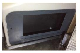
Sikaflex new BreatheSafe HEPA return air backing plate into place.
