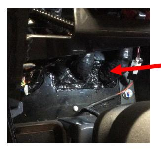
Seal around wiring glands / grommets.
