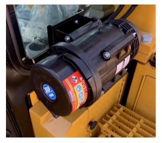
Ensure filter can be removed & system is easily accessible for servicing.
