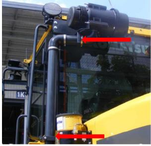
Secure ducting with brackets, stauff clamps.
