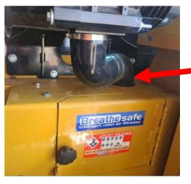
Example of ducting into OEM 3 inch fresh air inlet.
