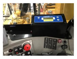
Solid mount controller in chosen suitable location by means of bolting / fixing in place.
