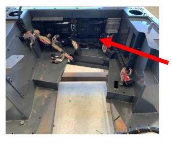
If applicable remove seat & internal panels to access potential air leakage points / run any wiring looms.
