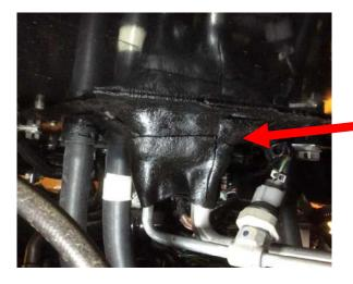
Seal around HVAC pipes / hoses.
