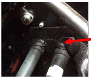
Seal around heater pipes / hoses.
