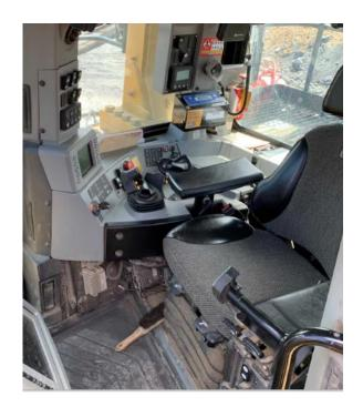
Refit inner console assy. Ensure all bolts are in place through floor to avoid leakage.
