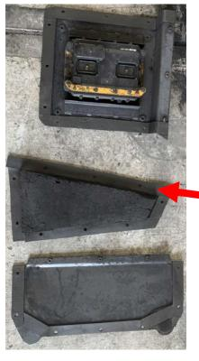
Apply sealing measures to accessible leak points & open glands.
