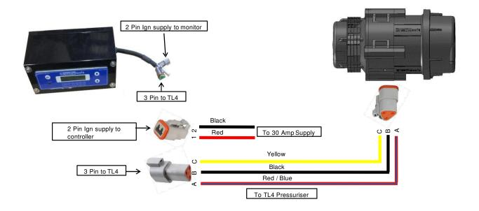
Follow pressuriser wiring connections as per the diagram. Upgrade the OEM pressuriser circuit fuse & use existing pressuriser circuit to power the BreatheSafe system.
