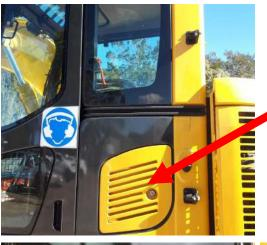
Locate the OEM fresh air filter inlet.
